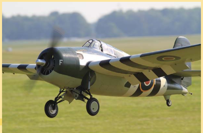
Mike Barbee's FM Wildcat designed by Bob Patton, on final approach with its flaps and gear down. The model is powered by a Moki .250 radial engine and weighs 90 pounds.
